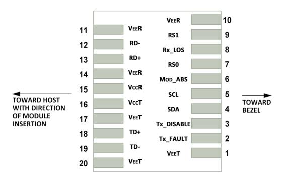
Host PCB SFP28 Pad Assignment Top View
